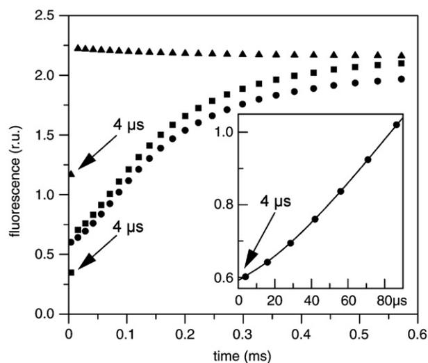
Fig. 1. Correction of the fluorescence changes by the instrument function. The instrument function (triangles) is obtained by submitting a fluorescent dye to the same illumination as the sample. Dividing the fluorescence changes measured with the sample (squares) by the instrumental function corrects for the variation in light intensity as shown with the circles. The inset shows a zoom on the early fluorescence changes after correction and illustrates the time resolution of the set-up.
