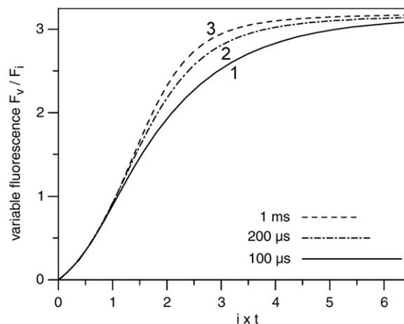
Fig. 4. Fluorescence increase measured from a young spinach leaf in presence of DCMU (40  $\mu\text{M}$ ) as function of the light intensity on a linear scale. Curves 1–3 same as curves 1–3 in Fig. 3.
